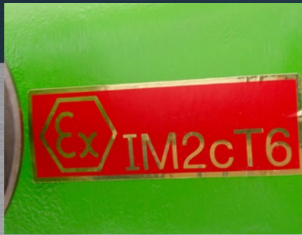
ATEX-Safety class approved as well for underground mining (coal mining)
