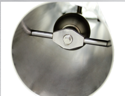
Suction side with venturi nozzle
